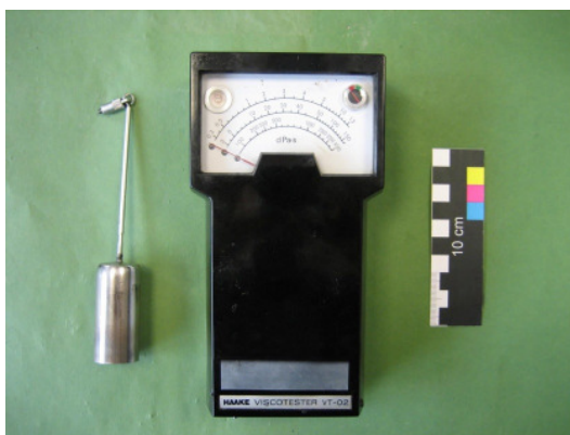
Fig. 1: View of a rotation viscometer (Viscotester VT-02, from HAAKE) with the appropriate hollow rotating cylinder of type 1 ( d_o \approx 24 mm, d_i \approx 22.5 mm, h \approx 53 mm)
